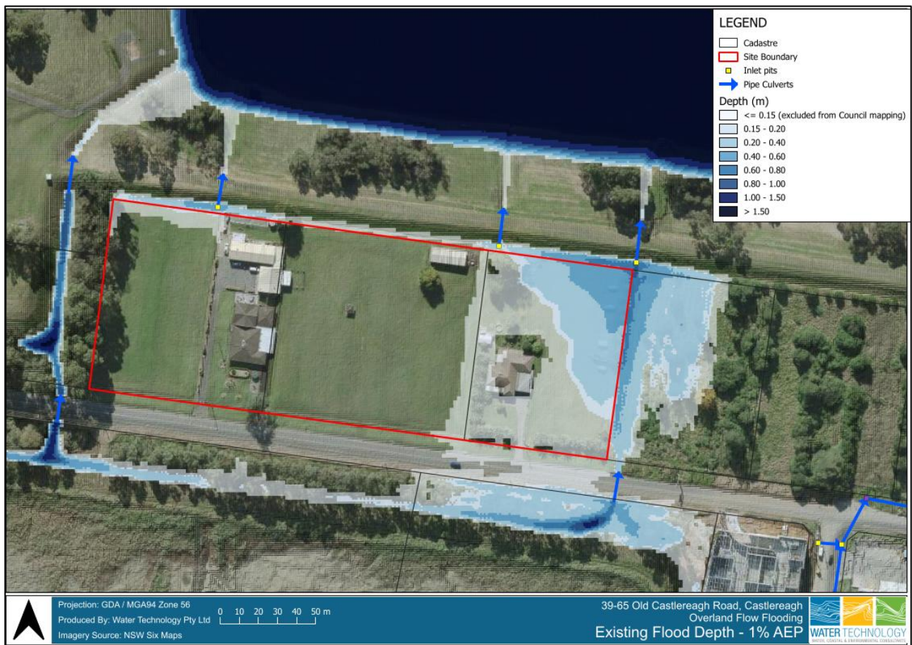
Figure 2-2 1% AEP Peak Flood Depth - Existing Conditions
